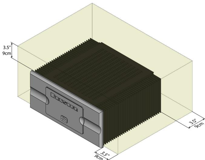
*Minimum recommended clearance for heat dissipation*
