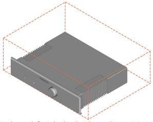
3.5 inches to left, right, back sides and top minimum recommended clearance envelope for effective heat dissipation
