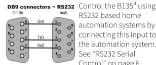
RS232 based home automation systems by connecting this input to the automation system. See "RS232 Serial Control" on page 6.
