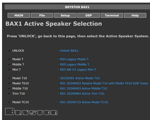
This interface will load showing all the current software available for specific Bryston **ACTIVE** speakers.
