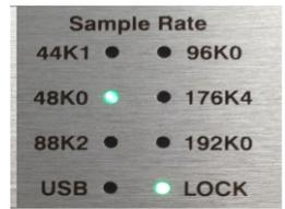
If the DAC does receive lock at any point during initialization then the Linux OS is starting up and loading drivers, this tells us the most likely culprit is a loose serial cable. You should check to make sure that the serial cable that connects the main-board to the microprocessor is connected and there aren't any loose wires.
