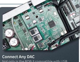
Not only is the BDP-3 compatible with USB and HDMI DACs but also DACs with traditional digital inputs. Use our S/PDIF or AES/EBU outputs and enjoy the benefits of our proprietary Integrated Audio Device. Measured jitter is so low it's nearly undetectable even by our state-of-the-art laboratory.
