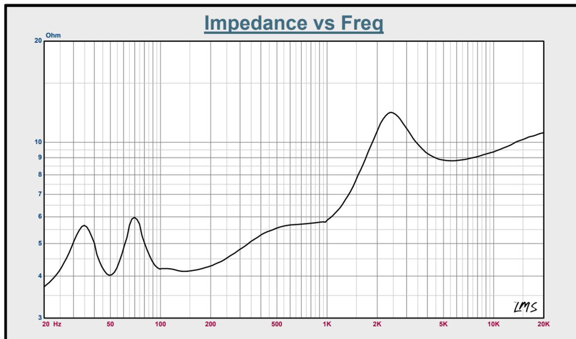
According to IEC/EN 60268-5 the nominal impedance (or more correctly the rated impedance) is to be no greater than 1.25 times the minimum impedance within the pass band.
