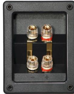
There are two gold-plated metal straps linking the two pairs of binding posts. Leave the metal straps in place (unless you are planning to bi-wire or bi-amp; see page 3) and use one pair of posts to connect your positive and negative (red and black) ends of the speaker cable. It doesn't matter which pair you use. Just be sure the gold links between the two pairs of binding posts are secure when you tighten the posts on the speaker connectors.
