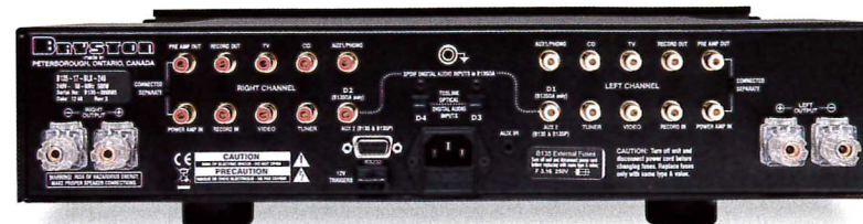
ABOVE: A full complement of analogue inputs and home integration connections, digital inputs pre-fitted awaiting the optional DAC module. But no USB provision
